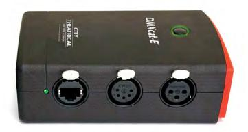
As the modern lighting industry evolves, there is an increasing need for test tools that include not only DMX and RDM capabilities, but also various ethernet protocols. As lighting manufacturers implement RDM Net, sACN, Art-Net, and other ethernet protocols, the  $\mathbf{DMXcat-E^{m}}$  is an essential tool for the future of lighting.
